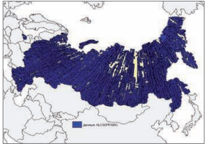
Fig. 8 – This map shows the coverage of Russia that has been acquired by the PRISM three-line pushbroom stereo-scanner which is mounted on the Japanese ALOS satellite. (Source: Sovzond)
