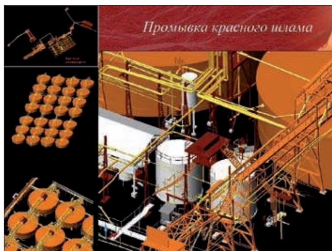
Fig. 10 – Showing some of the CAD drawings of the Friguia aluminium refining plant in Guinea, West Africa that have been derived from a ground-based laser scan survey. (Source: Jena Instrument)
