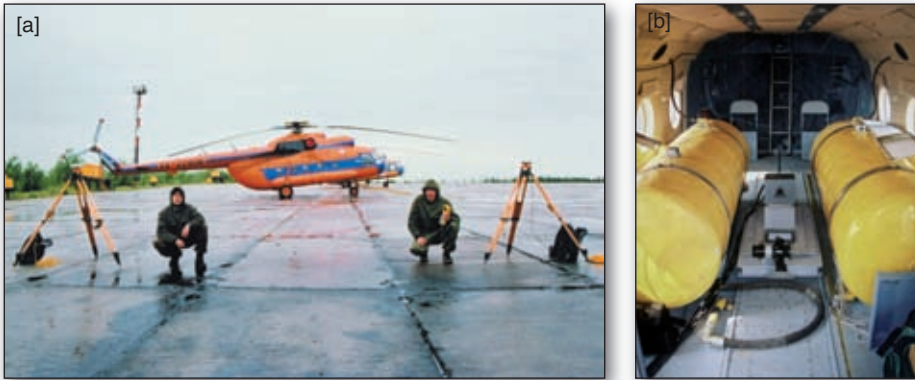
Fig. 2 (a) - A large Russian-built Mil-8 helicopter used as the platform for an Optech ALTM airborne laser scanner. In the foreground are the tripod-mounted antennas of the Trimble 5700 GPS receivers that are used as the ground-based stations for differential GPS positioning of the helicopter during its flight operations.
